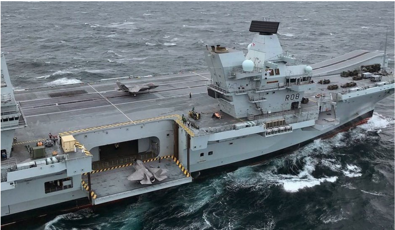
Above: Forward lift on HMS Queen Elizabeth with F-35B's on the lift and the flight deck
